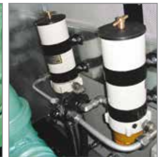
▲ TWIN-Filter Wasserabscheide Twin water separator filter
