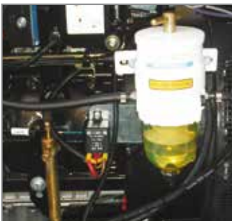
Wasserabscheider Typ Racor Water separator filter Racor type
